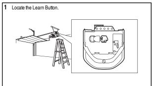
Press and immediately release the Learn button. The Learn LED will glow steady for 30 seconds. Within 30 seconds...
